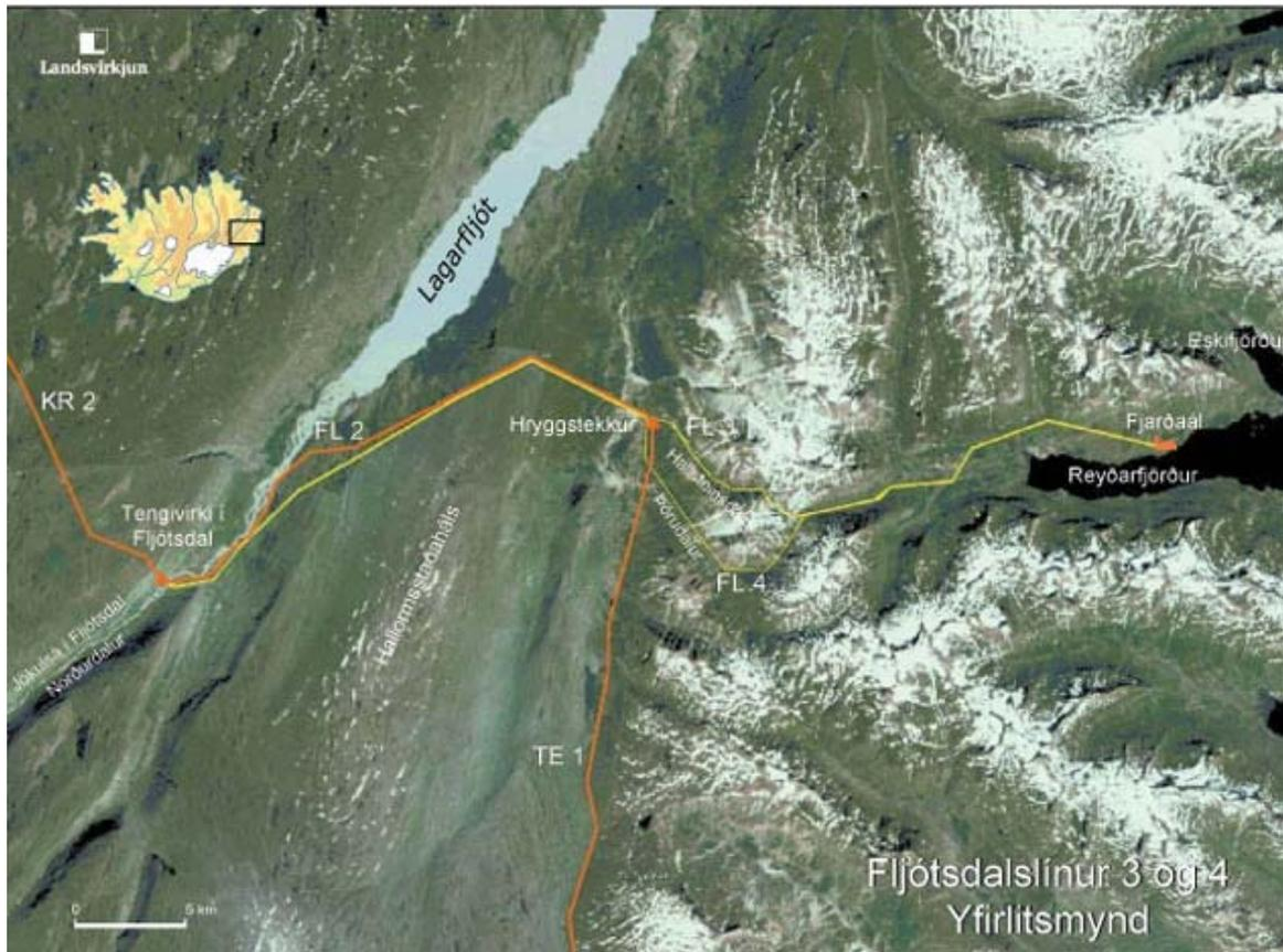
**Figure A-3. Graphic Representation of Fljótshérað Transmission Lines**
